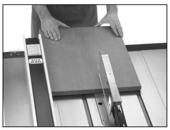
Figure 37. Do not stand directly behind wood!
